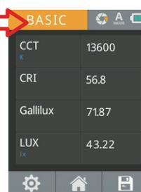
Basic mode (after measurement) Press the capture key again to see the measurement results.
