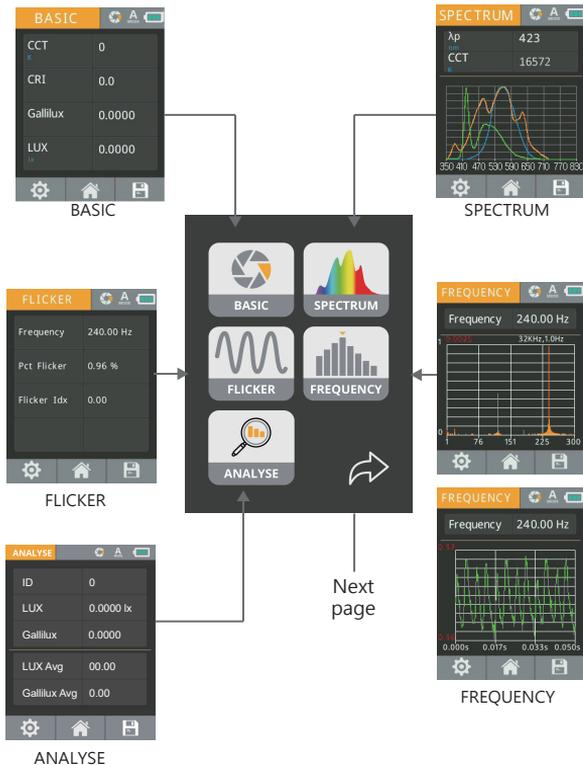
The analyse button allows you to analyse the data of a defined number of measurements.
