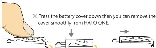
※ Press the battery cover down then you can remove the cover smoothly from HATO ONE.
