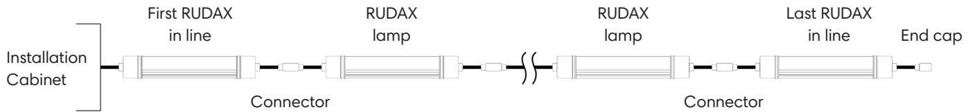
See data sheet for amount of RUDAX installed in one line.
