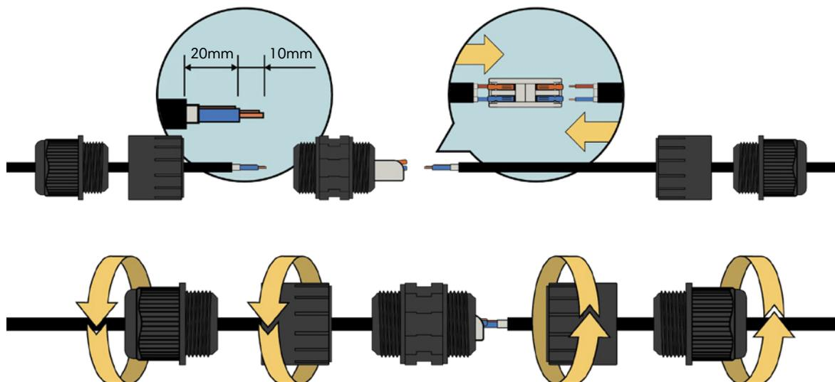
**Note:** For a connection with round cables, the specific round rubber needs to be placed inside of the gland.
